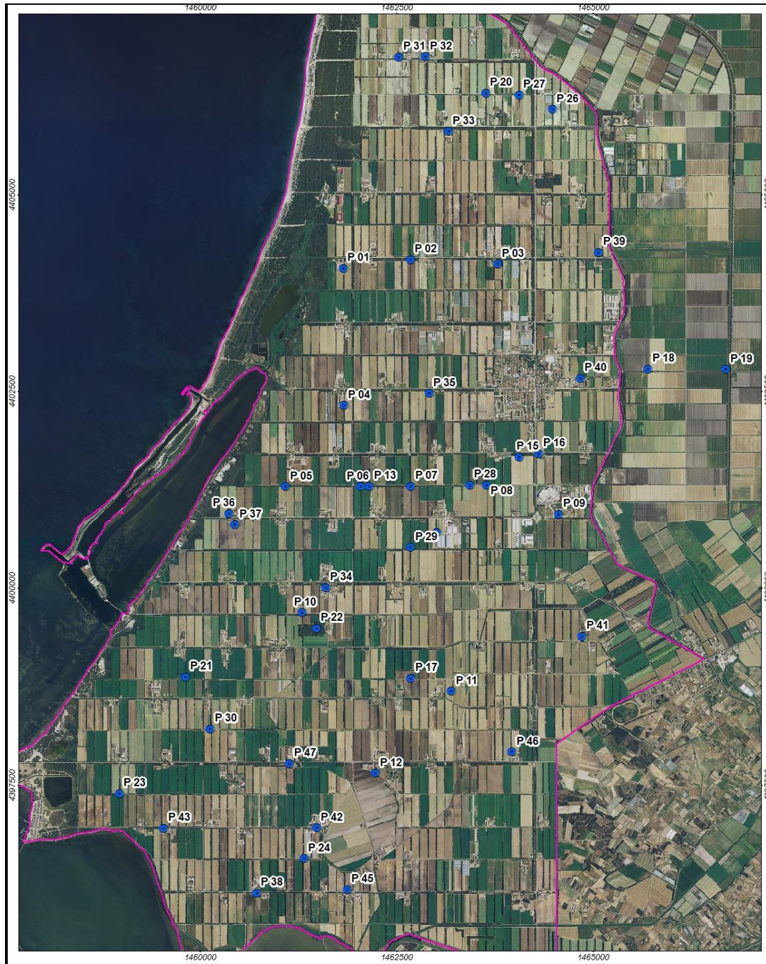
Fig. 1 - Groundwater monitoring net stations in the Arborea plain.
