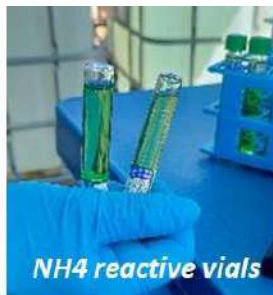
Kit measurement range: 12.5 - 130 mg/L of ammonia
