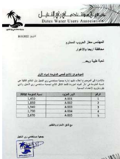
Fig.13 Salinity of ground water of the 5 wells which feed the strategic water project of DWUA. All 5 wells show from moderate to severe salinity
