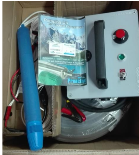
Image 2 – Pump for piezometer purge
