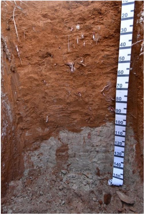
Fig. 20- Soil Type 4: the greyish-whitish lacustrine material at about 100-120 90 cm deep (P4, 2022)
