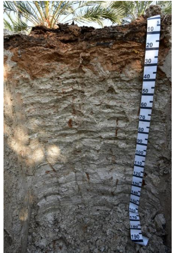
Fig. 23 Soil Type 7: representative profile, with 30 cm deep alluvial DEPOSITS (P3 2022)
