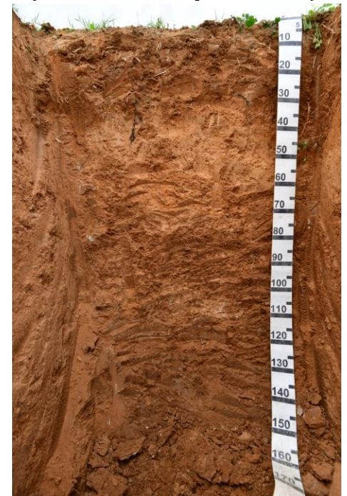
Fig. 19 Soil Type 3: in this profile the alluvial deposit is very thick, and the lacustrine material was not reached (P12, 2022).
