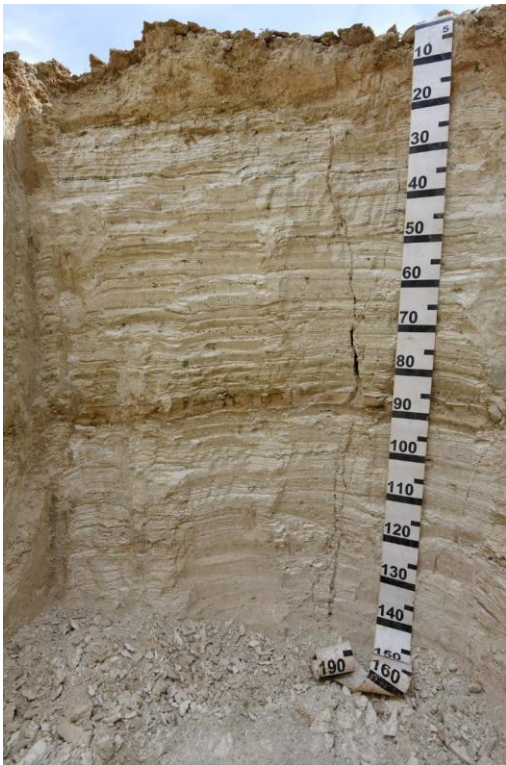
Fig. 21 Soil Type 5: see the fine horizontal stratification of lacustrine deposits (P9, 2022), the gypsum crystal layers and the salt crust on the surface
