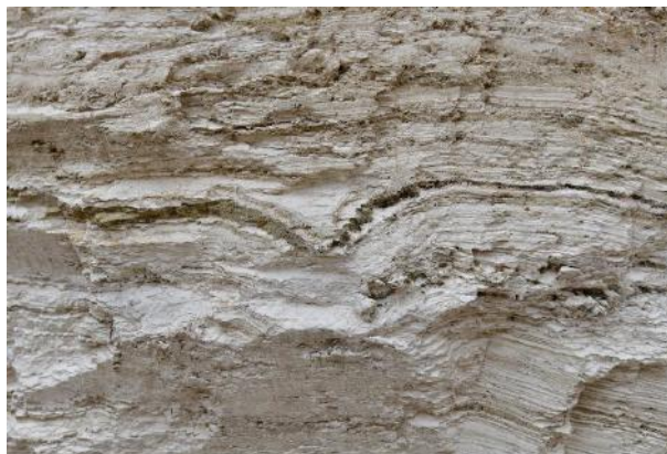
Fig. 21 Soil Type 5: see the fine horizontal stratification of lacustrine deposits (P9, 2022), the gypsum crystal layers and the salt crust on the surface
