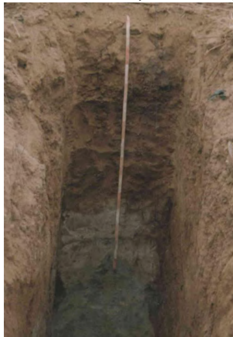
Fig.18 An example of Soil Type 2: the two parent materials are very evident: the alluvial deposit in the upper part, the lacustrine in the lower part
