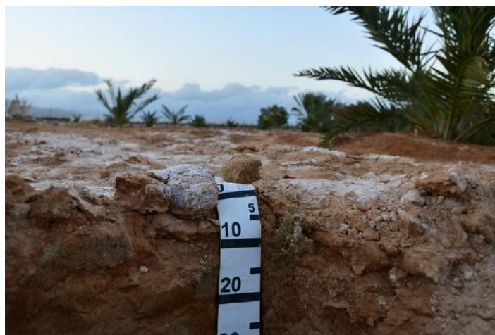
Fig. 22 Soil Type 6: A broken the petrocalcic/petrogypsic horizon starts from 40-60 cm deep; petrogyptic horizon fragment and surface salt crust (P14 2022)
