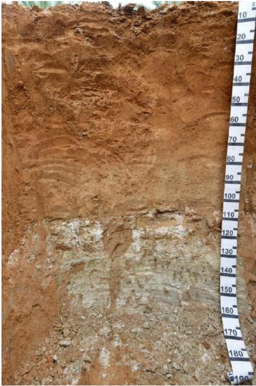
Fig.17 c - Soil type 1, and P7, with its salty crust
